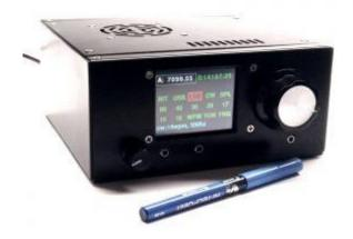
The sBitx is a kit radio you can assemble with a screwdriver and a pair of pliers. Next month, we'll dig into the sBitx further. For now, here's a list of the HF transceivers features:
