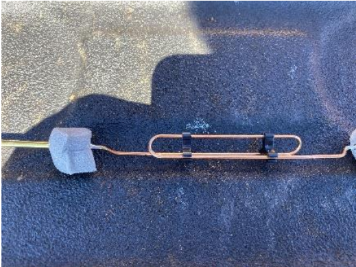
Figure 2 One of several collinear stubs inside the antenna
